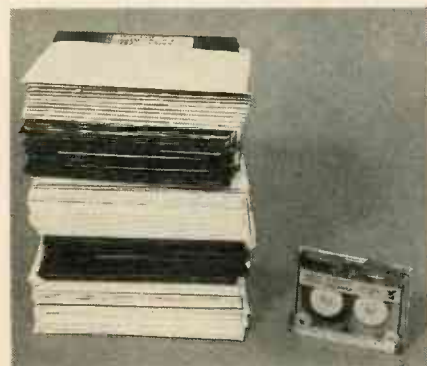
WHICH WOULD YOU RATHER USE to back up 30 megabytes of data? The stack of ninety disks on the left can do it, but the DC-2000 cartridge makes it more likely that you'll actually get it done.
