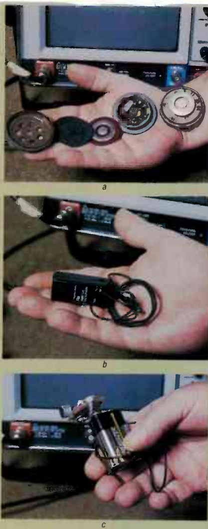
FIG. 1—THESE ARE CLANDESTINE radio bugs. In (a), a parasitic phone-tap is shown disassembled. In (b), a Radio Shack FM-transmitter (part No. 33-1076) can be conveniently dropped behind the cushion of a chair. In (c), this tiny FM transmitter can be hidden in a kitchen cabinet.
